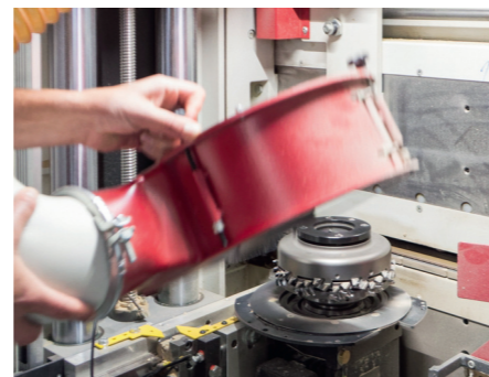
To reposition the cutting edges, the dusthood must be released
