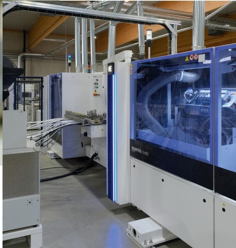
The nesting lines transfer to the edgebanding lines visible in the background
