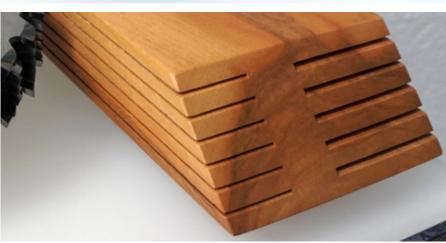
By using Leitz thin-cut circular sawblades, for example, 7 instead of 6 slats can be produced. This means an increase in productivity of about 17 %.
